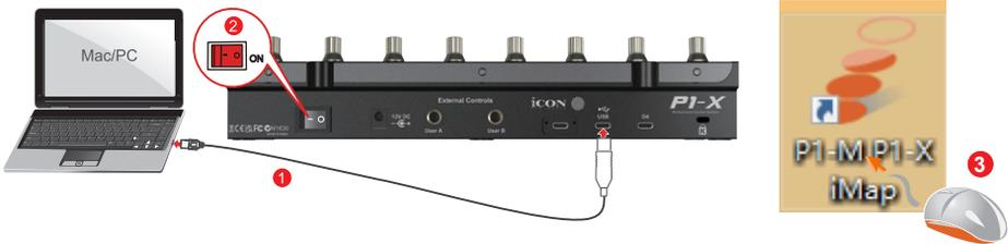
**Step1:** Connect the P1-X using a USB C connection. Press the “MIDI Device” button at the top to select your connected P1-X as the “MIDI In and Out” device in the pull-down menu?
